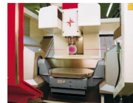
Integrated laser light barriers for high precision toolpiece measuring and broken toolpiece identification
