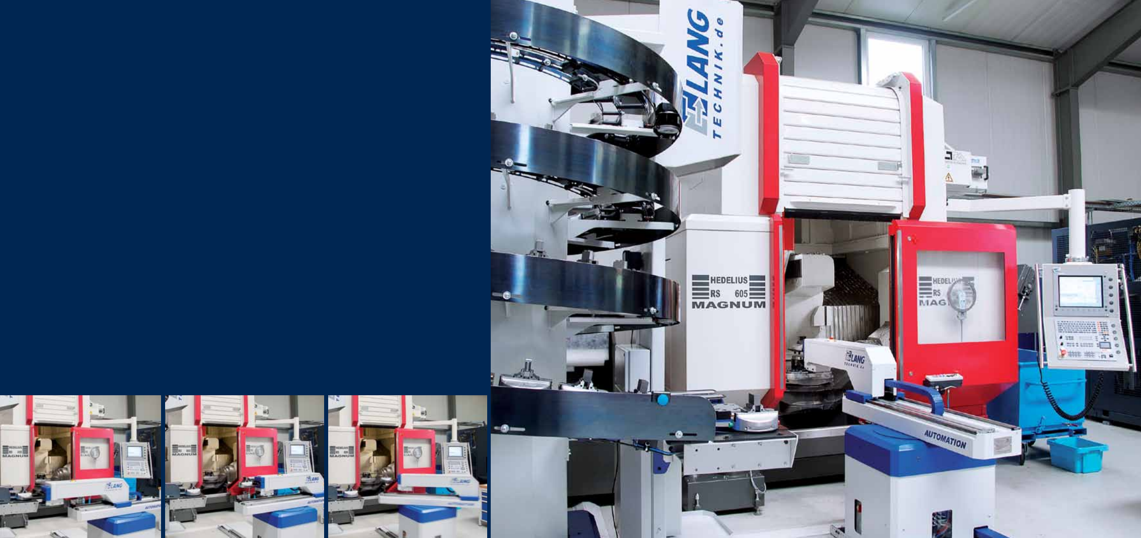
The HEDELIUS RS 605 was fitted with cutting-edge automation technology by Lang. Loading with workpiece pallets is fully automated.
