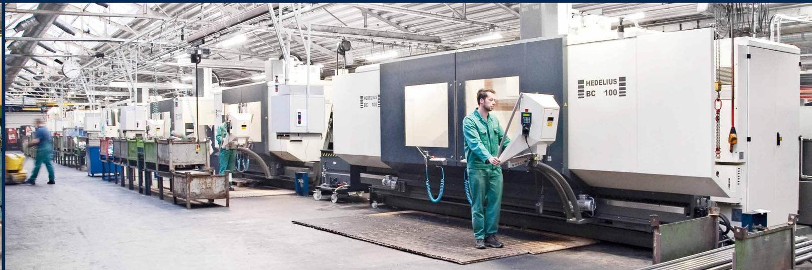
The Krone engineering company was able to increase its productivity even further with the HEDELIUS BC 100. The machining centre has a travel path of 2500 or 3500 mm depending on the model.
