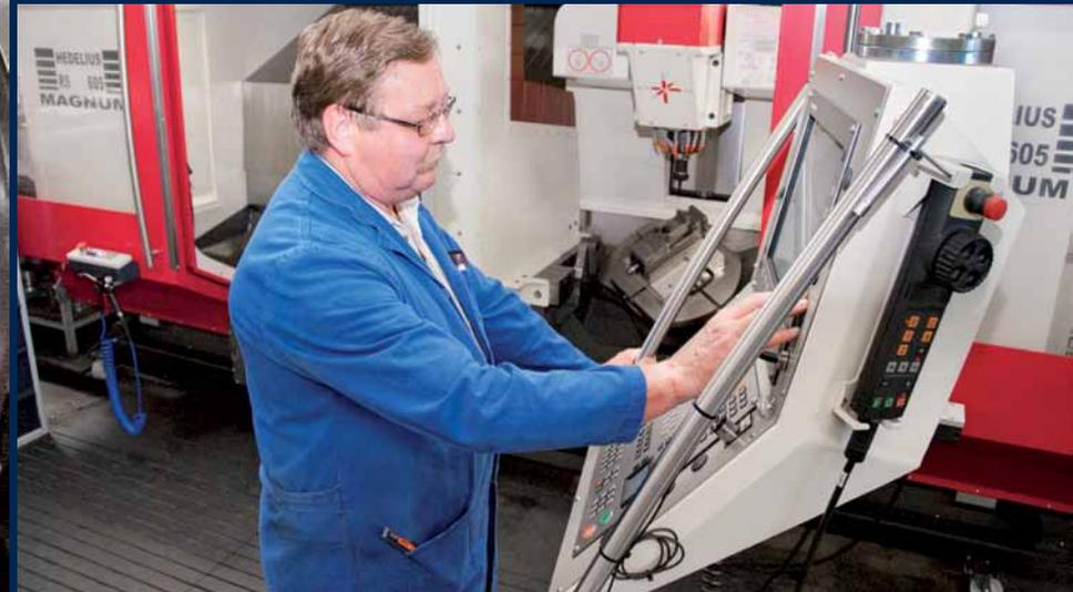
The main spindle of the HEDELIUS RS 605 has an output of 165 Nm/18.5 KW and a maximum speed of 8000 rpm.
