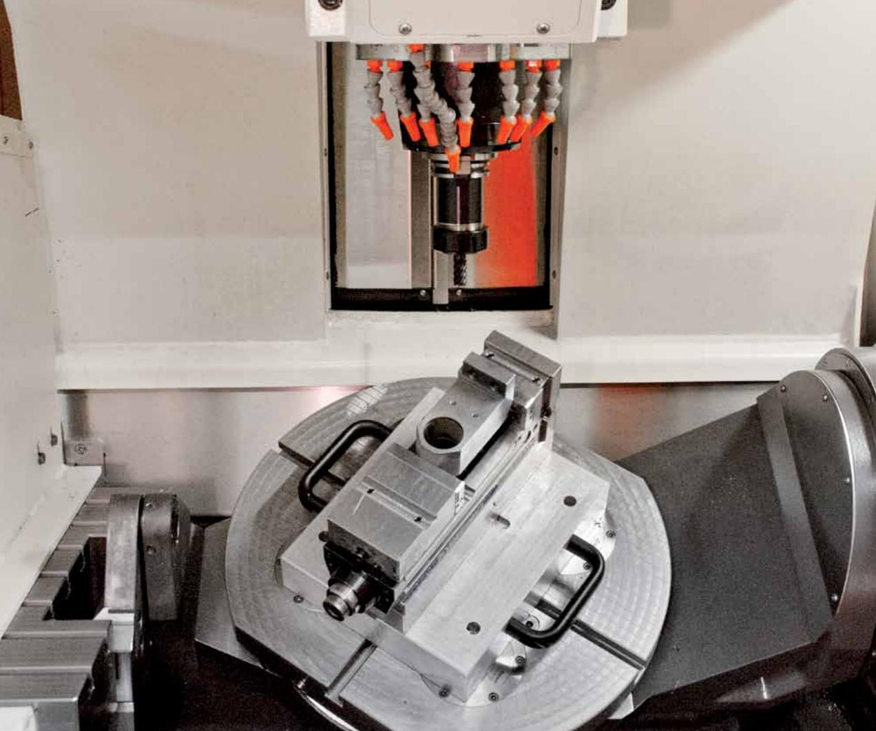
Milling mechanic Armin Sobisch says, „The RS 605 with zero-point clamping system is ideal for small series.“
