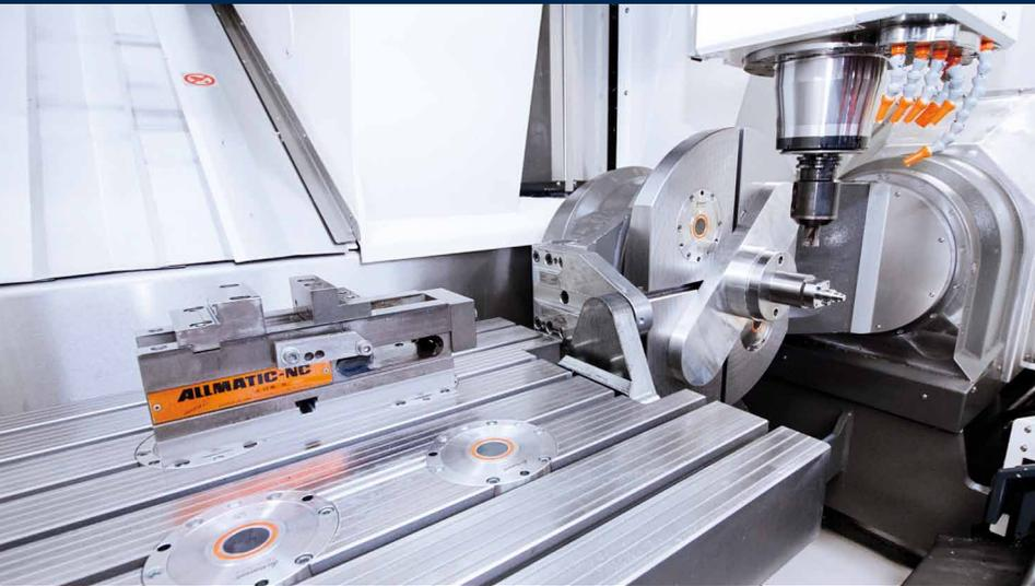
In the fixed machine table and the swivel table of HEDELIUS RS 605 K IC four clamping cylinders each are integrated.
