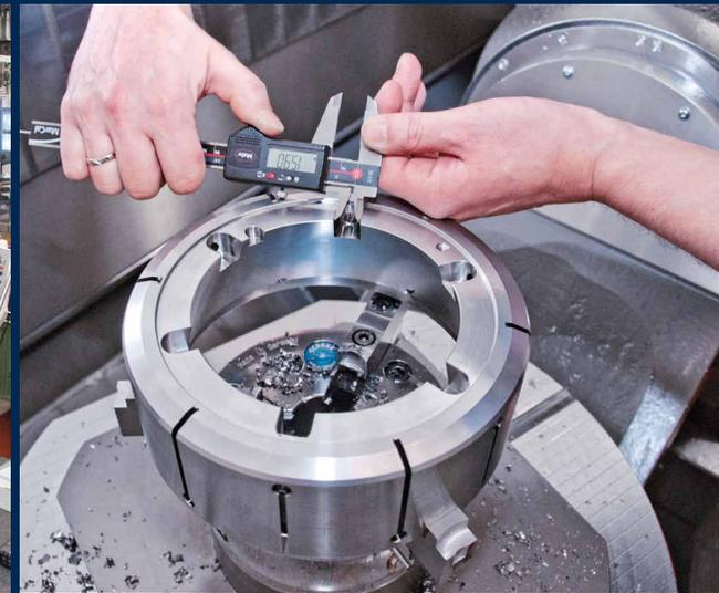
The swivel table of RS 605 is ideal for 5 and 6-sided machining of complex workpieces.
