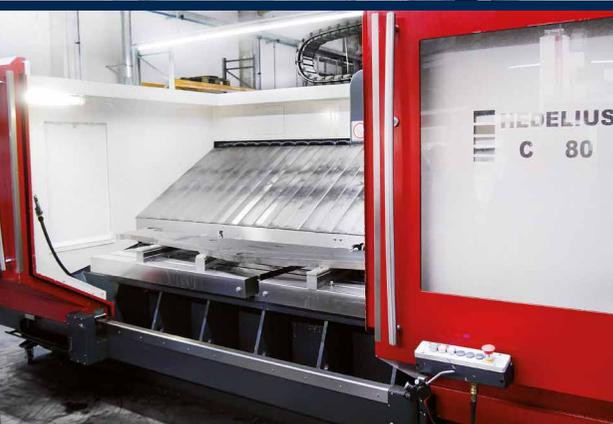
BL-Lasertechnik's first machining centre. Parts for welded assemblies are mechanically processed on the C80 2300.
