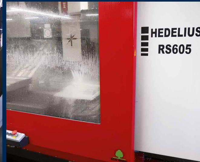
The RS 605 K20 is mainly used for machining aluminium, while the robust machine table and rotary table significantly reduce the set-up requirements.
