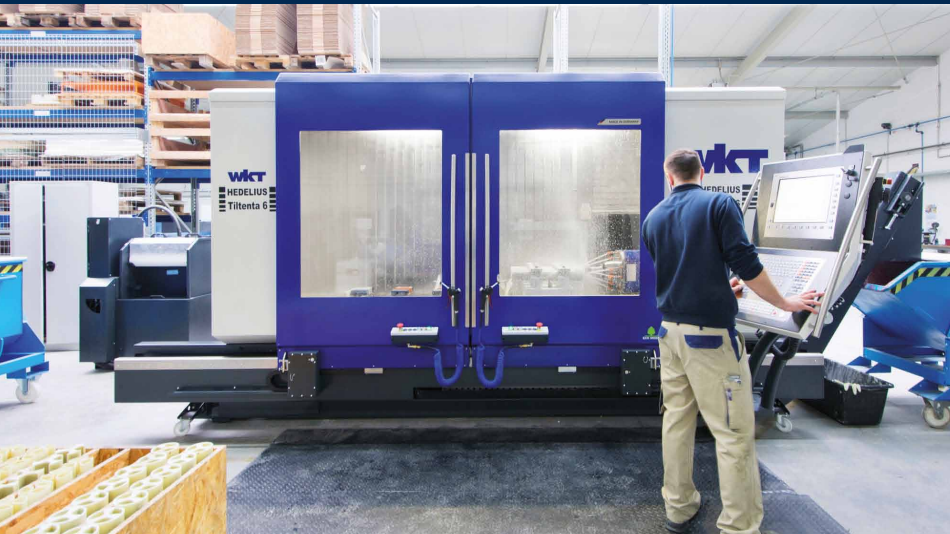
The material GRP is sometimes used in heavy-duty machining operations and processed here on the swing-spindle machining centre Tiltenta 6 2300.
