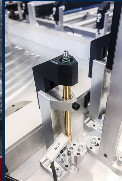
Sensor mountings with a cover from Zander EMS, used for special machinery for the automobile industry.
