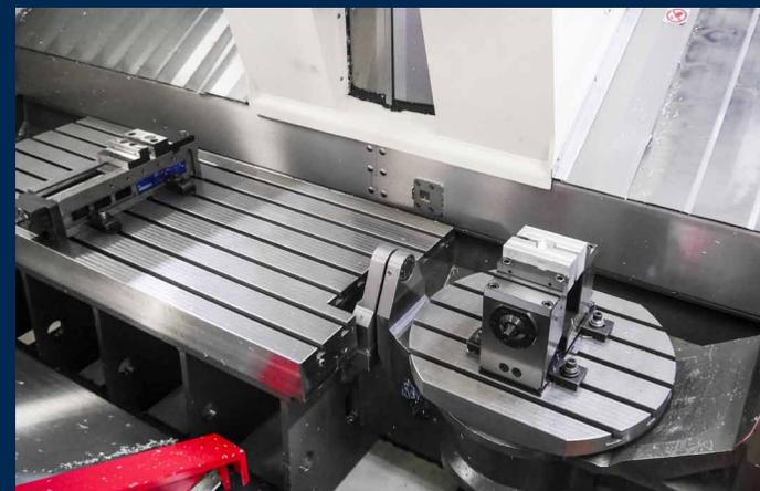
With its rotary tilt table and fixed machine table, the RS 605 K20 offers major flexibility in production.
